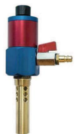
The ARIANA Power Vac Pump is a dual-acting suction and pressure pump that uses compressed air. It is mainly used for filling and emptying lubricant and coolant tanks. The pump was designed for fast and trouble-free installation at standard barrels. It is screwed into the bunghole of the barrel and connected to the compressed air supply. A feed hose is attached at the other barrel opening.
