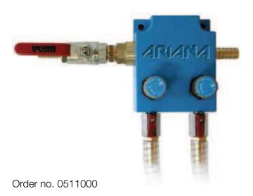
A mixing unit is essential for mixing emulsions and grinding solutions. By means of two needle valves, the ARIANA Duo Mixing Unit permits fast and precise adjustment of the emulsion concentration of liquid coolants and lubricants. In this way, it is possible to produce liquids using optimum concentrations.
